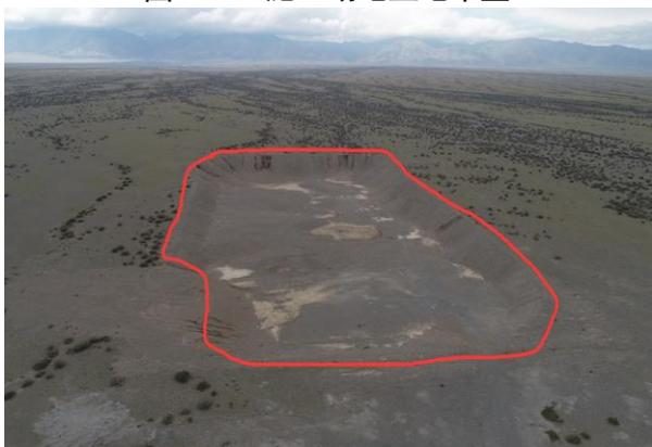
图4.1-7 取(弃)土料场削坡、土地平整
